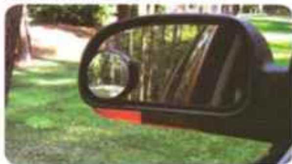
▲ Figure (8): The image that is formed by the convex mirror is virtual, upright and smaller than the object.
